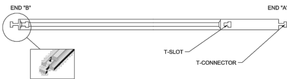
DETAIL 4: INDIVIDUAL FIBER-COMPOSITE BRACING BAR
